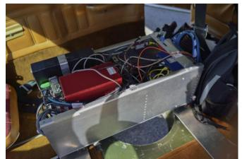
*G-LiHT sits inside the airplane's cockpit, over an open camera port that allows it to look down from about 1,000 feet high. Credits: NASA/Goddard Space Flight Center*
