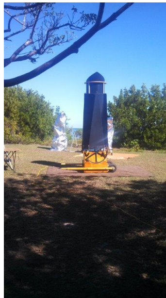
Mike Usher's Dobsonian mounted 20" f5 Reflector.
