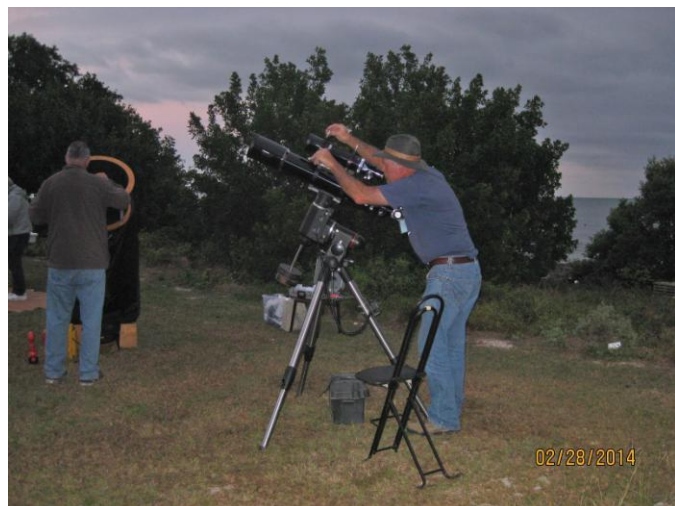
Rick Piper – Orion 80 mm Refractor f5, German Equatorial Mount. Setting up for imaging. Eric Uthus in background.
