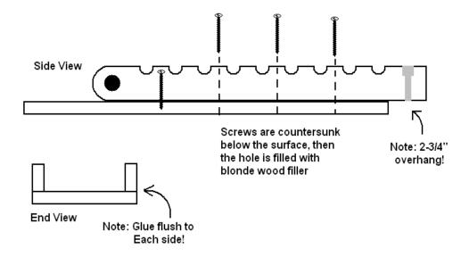
14. The next step is assembling the rear leg. Take the two identical pieces from step #7 (48" x 1.75" each), and the single piece from step #9 (42" x 2-7/16"). Clamp and glue as shown below. I do not use screws on this sub-assembly, because there is no shear force on this part, (all the weight is carried in compression.)
