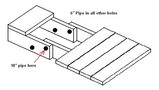
Insert the remaining 6" pipe into the 3<sup>rd</sup> hold drilled in the seat box in step #33. You can now hang the step box over the top of the close frame in its stored position, and lay the assembly flat on
